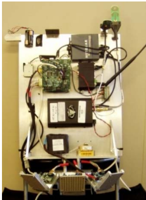
Figure 1: GLANSER GLU prototype, which is a backpack-mounted personal navigation system
