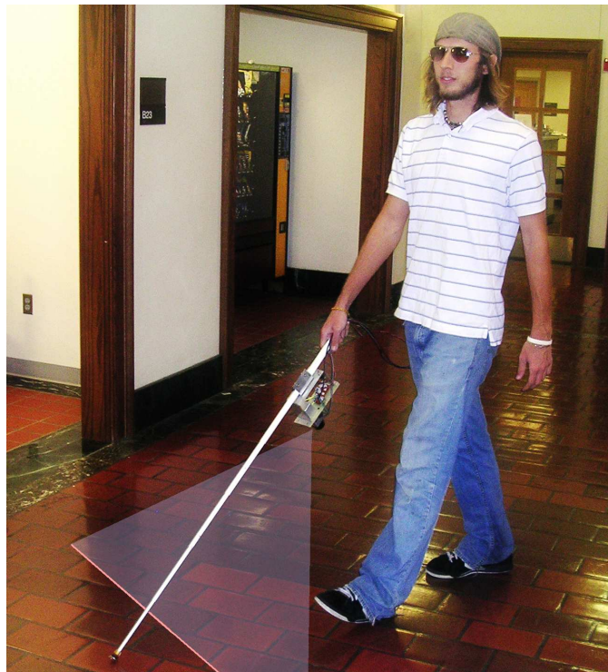
Fig. 1. This figure depicts the typical usage of our localization aid, which estimates the pose of a person walking inside a building. The sensing package is mounted near the handle of the white cane, and a portion of the 2D laser scan plane (60 out of the 240 degrees field of view) is illustrated, along with the line of intersection between the scan plane and the floor.
