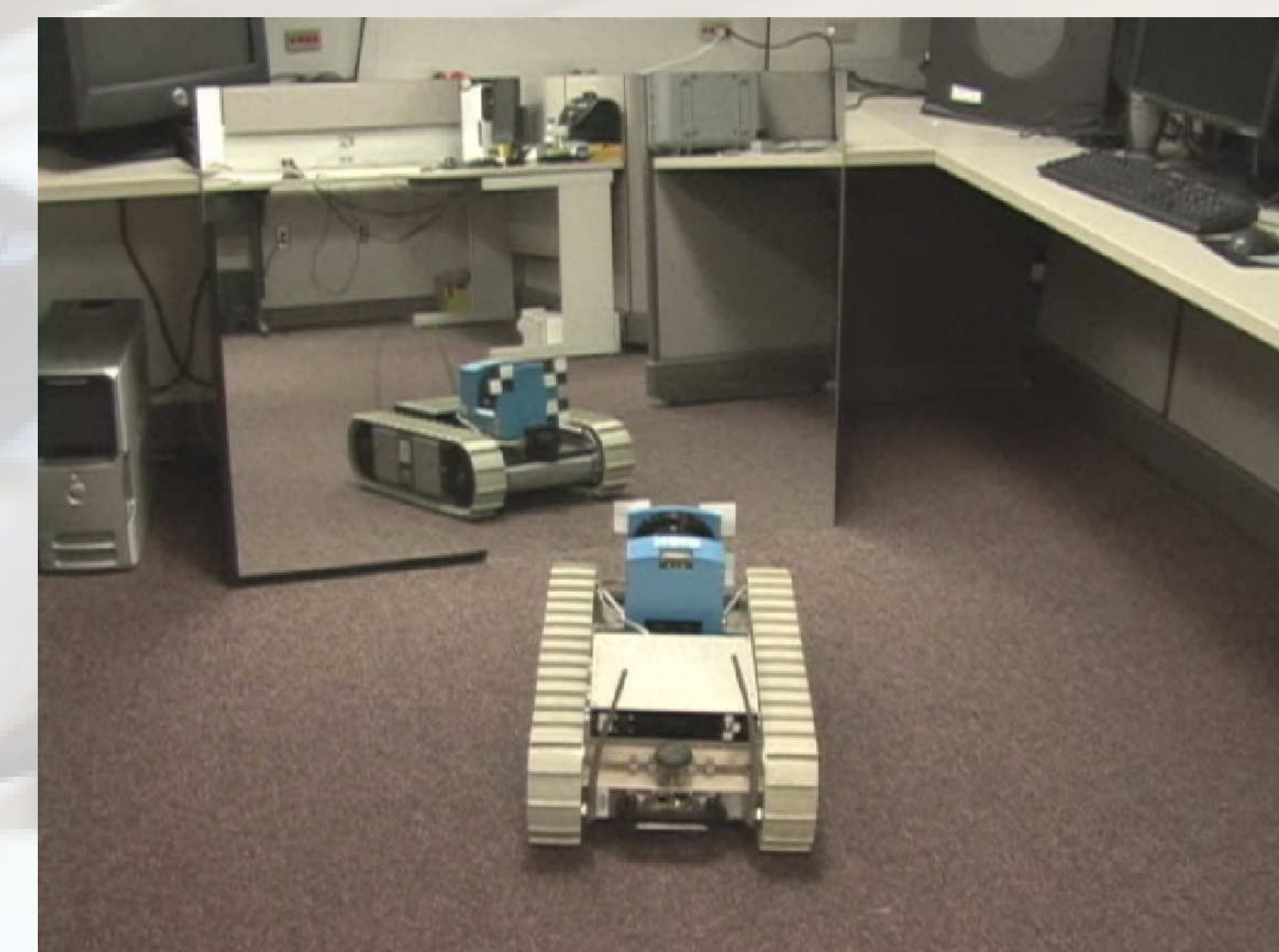
Robot moving in front of a planar mirror with 3 fiducial points attached on a laser scanner.
